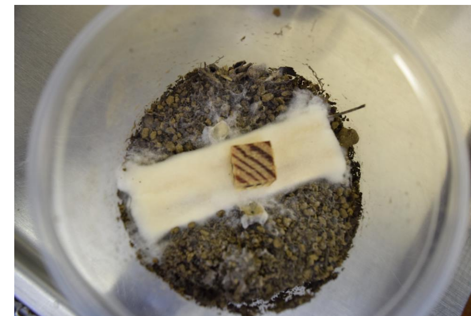
Figure 7. Example of decay resistance testing in AWPA E10 soil block study.
