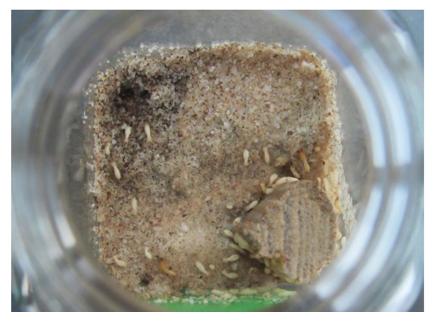
Figure 8. Example of termite repellency testing in AWPA E1 study.
