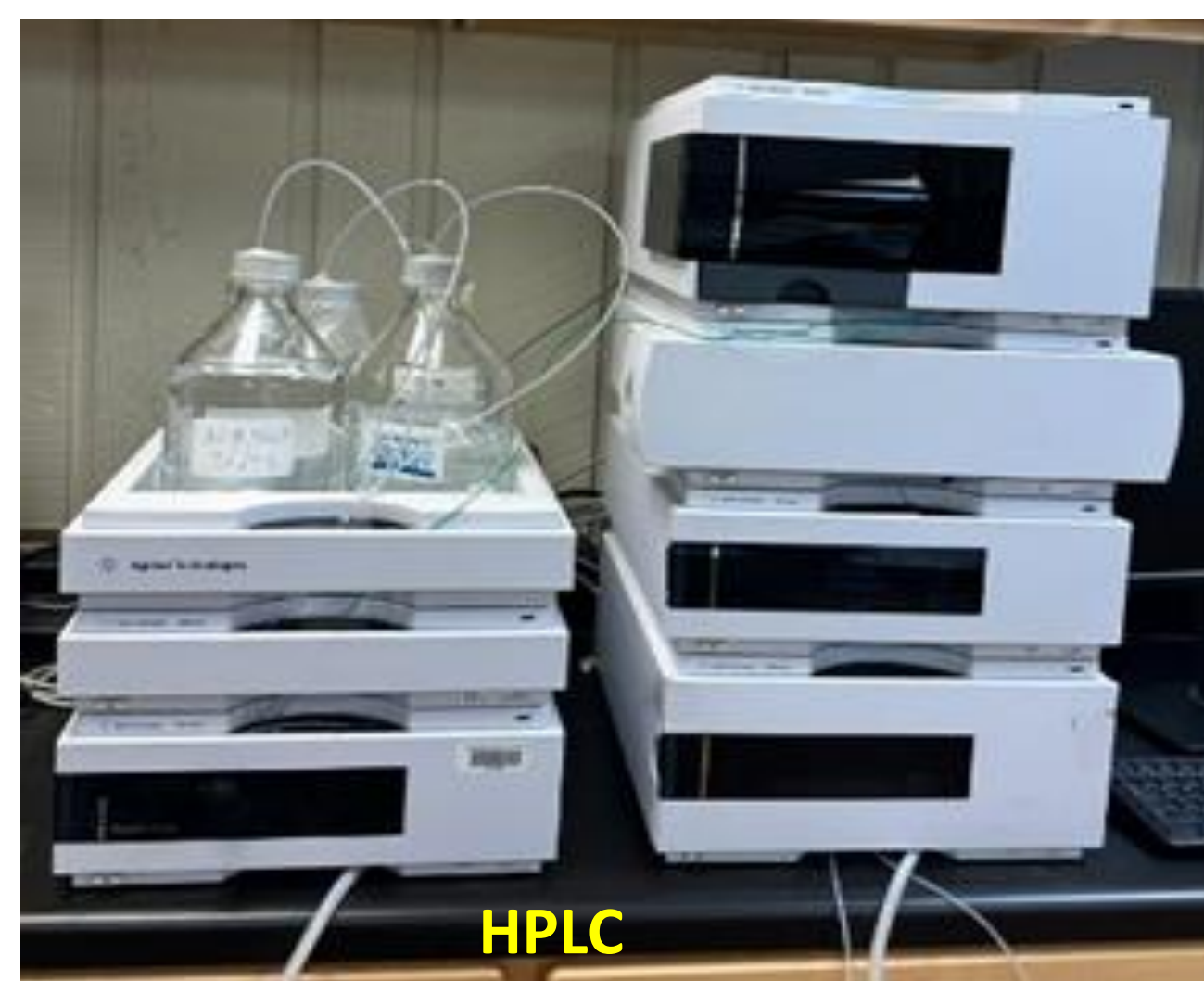
Figure 5. High Performance Liquid Chromatography (HPLC) uses a liquid chromatography system's stationary and mobile phases to separate, identify, and quantify mixture components.
