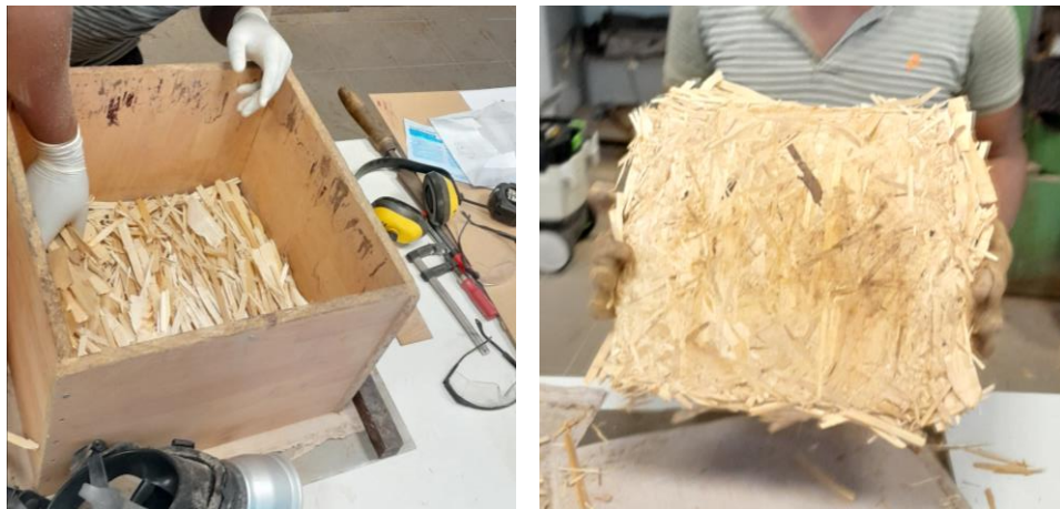
Figure 6 – Producing small OSL samples in the lab and the finished panel
