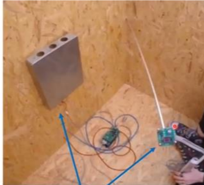
Convective heater and thermal comfort sensor
